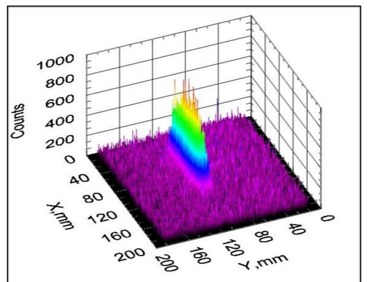
Fig. 5 spectrogram of a neutron beam passing through a limiting slit
