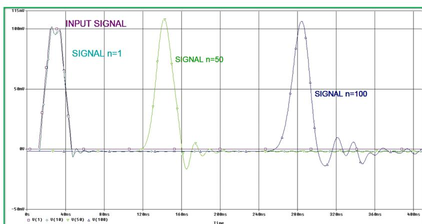
Fig. 3 Signal from the tap of the delay line N = 1, N = 50, N = 100
