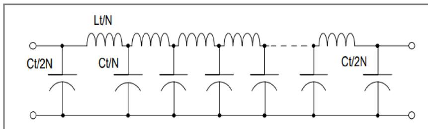
Fig. 2 Delay line circuit consisting of N number of LC circuits.
